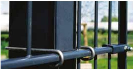
**Figure 7-6:** Bar grating fence with horizontal U-shaped profiles as endless fence with variable distances between posts
