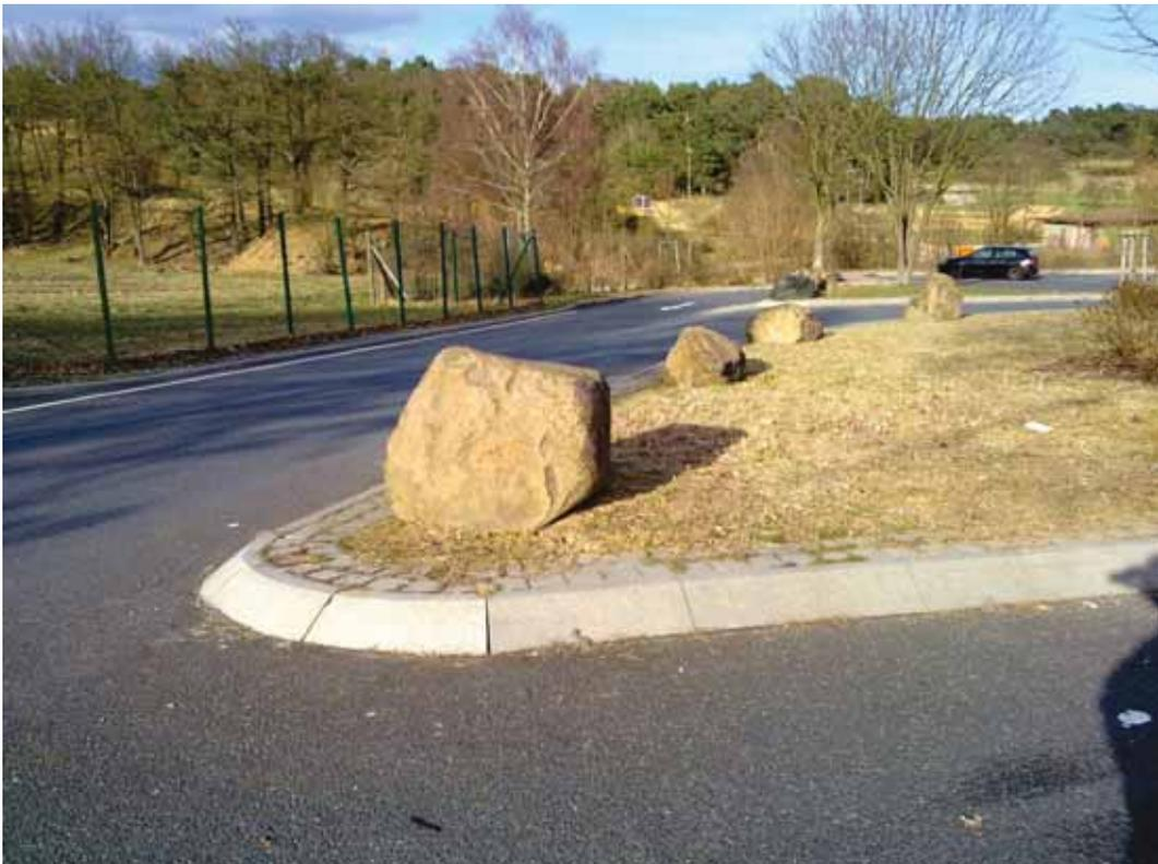
**Figure 7-2:** A serpentine access road prevents an attacking car from reaching a critical speed.
