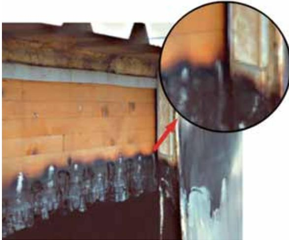
**Fig. 7.01:** No spread of fire inside the elements
