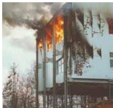
**Fig. 6.01:** A major fire experiment with sandwich elements as external components
